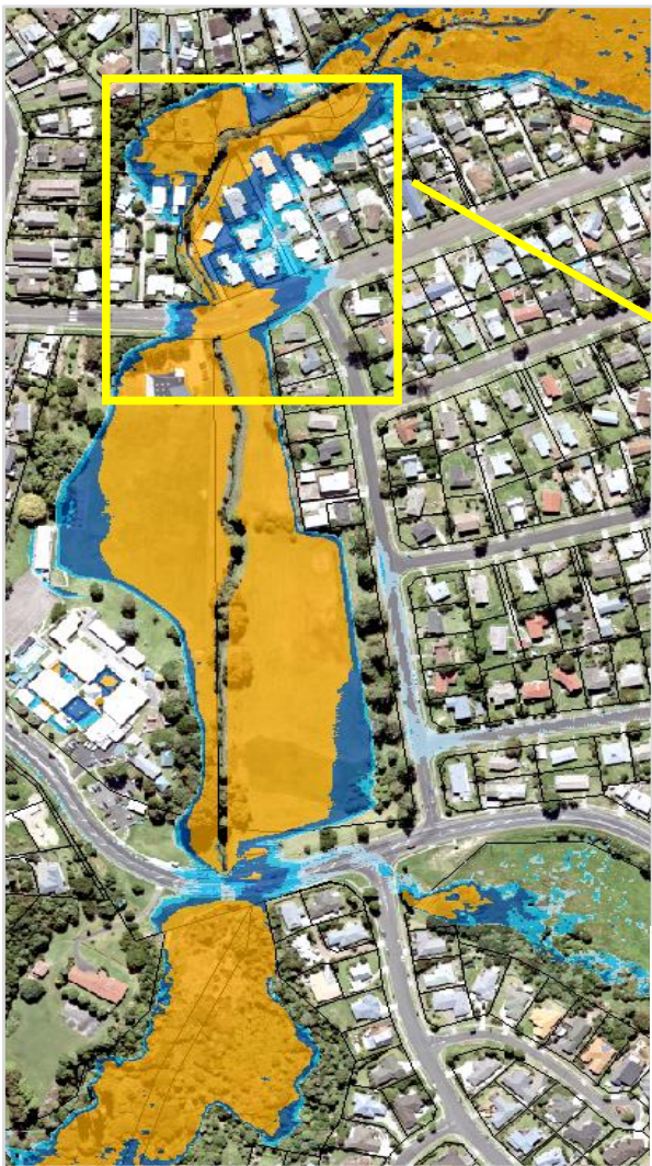
Left): 1 in 100-year Flood Hazard (flood depths (metre) indicated in key to bottom right)
