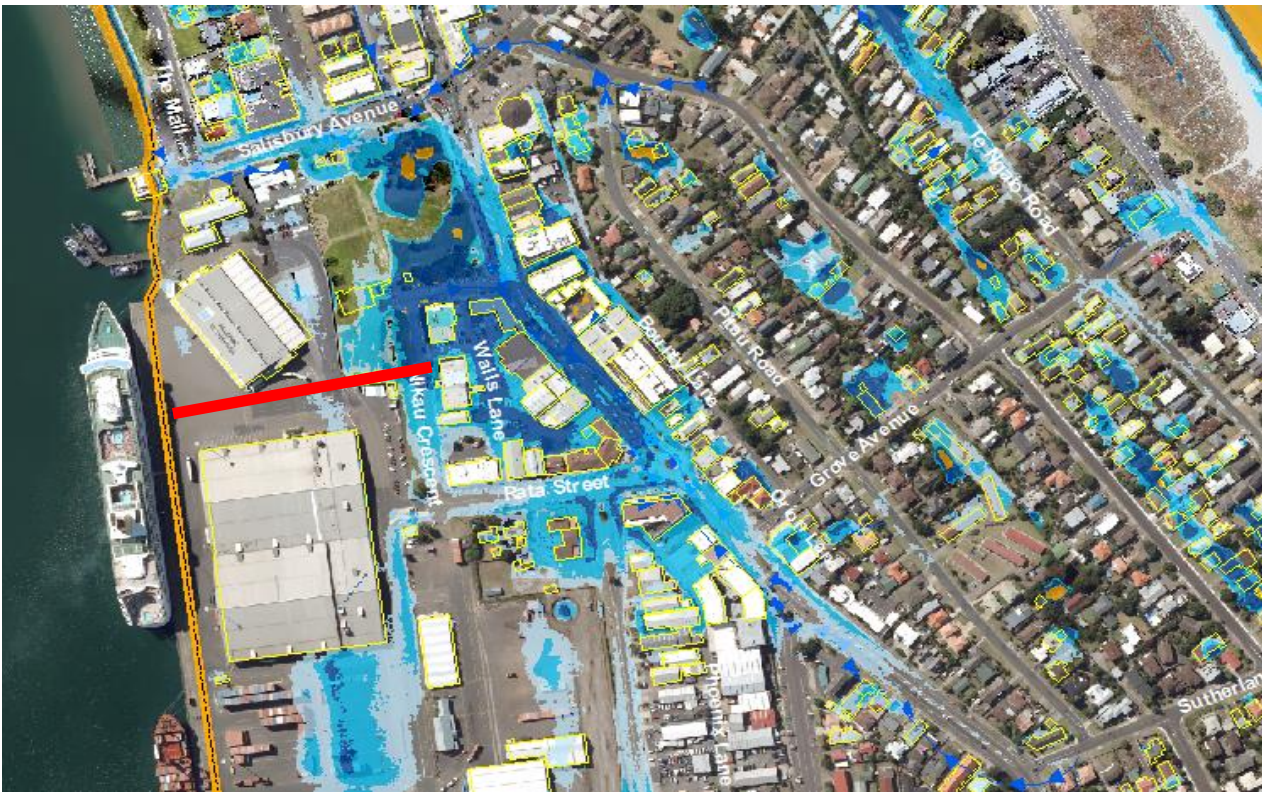
Left): Flood hazard map for Mount North in vicinity of outlet (indicative location denoted in red) Right top): Three sub-catchments which can be serviced by the new outlet Centre) During outlet construction (late 2017/2018) Right bottom): Outlet alignment through Port of Tauranga
