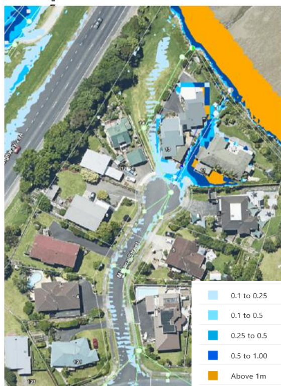
Left): 1 in 100-year Flood Hazard (flood depths (metre) indicated in key to bottom right)
