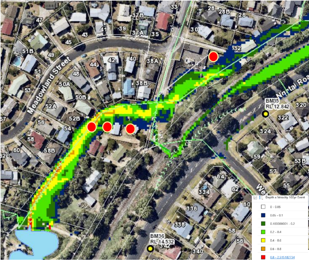
Above) 1 in 100-year Flood Hazard (flood depths (metre) indicated in key to bottom right). Red dot/dash indicate properties/land purchased. Overland flowpath extent roughly denoted by yellow dashed lines
