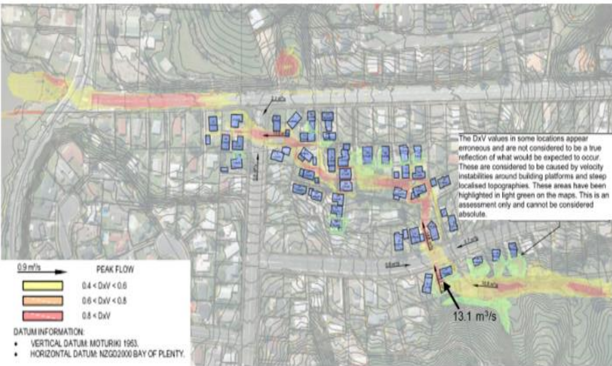
Figure 2: DxV flood hazard (yellow, orange and red all indicate flows in excess of Council's LoS threshold for intervention – yellow \geq 0.4 \text{ m}^2/\text{s} , orange between 0.6 - 0.8 \text{ m}^2/\text{s} , and pink \geq 0.8 \text{ m}^2/\text{s} )
