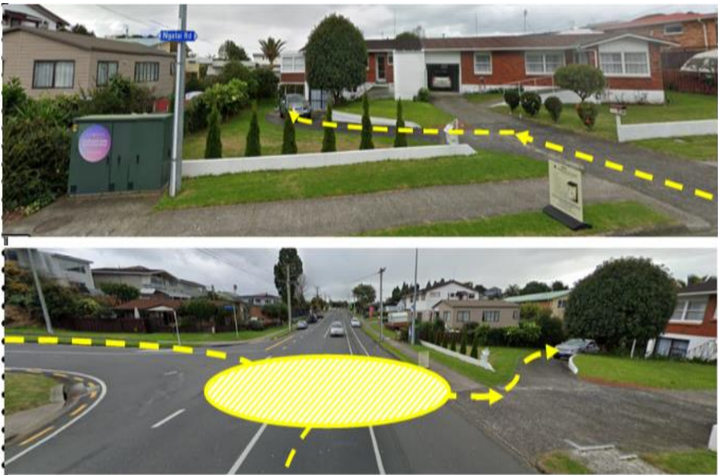
Upper and Lower: 247B Ngatai Road, yellow hatch and arrows show ponding and direction of overland flow from Freyberg Street and Ngatai Road overtopping driveway and passing down side of property
