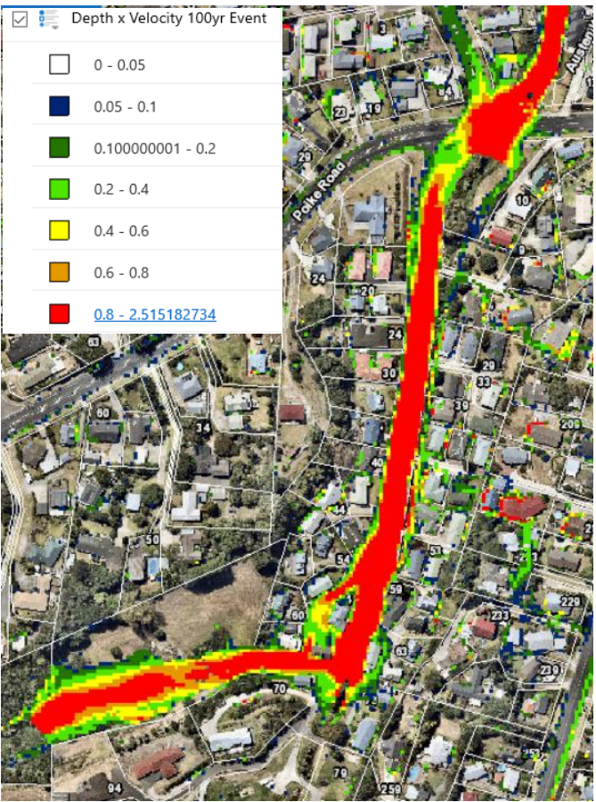
Above) Awaiti Place and surrounds1 in 100 year DxV flood hazard – yellow and red above 0.4m 2 /s threshold. 105 properties either directly impacted with flood waters through dwelling and/or land, or access from property onto Awaiti Place severely compromised
