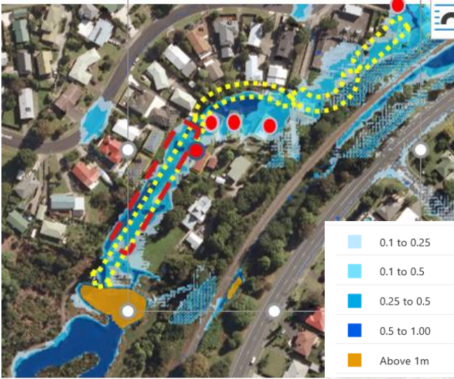
Above) 1 in 100-year Flood Hazard (flood depths (metre) indicated in key to bottom right). Red dot/dash indicate properties/land purchased. Overland flowpath extent roughly denoted by yellow dashed lines
