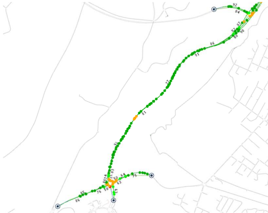
Figure F2 Preferred with Peak Spreading - 8:30am congestion at Takitimu & Tauranga Crossing
