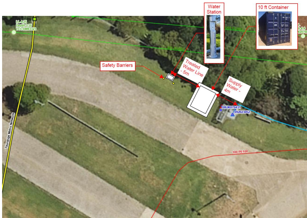
Figure 2: Concept Layout of the Fluoride Removal System
