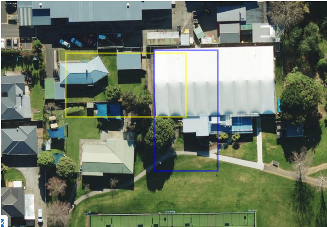
Figure 6-1: Two alternative footprints which minimise exposure to the infilled gully and slope edge. These are provided for discussion only, and consideration of land procurement is beyond the scope of this work.
