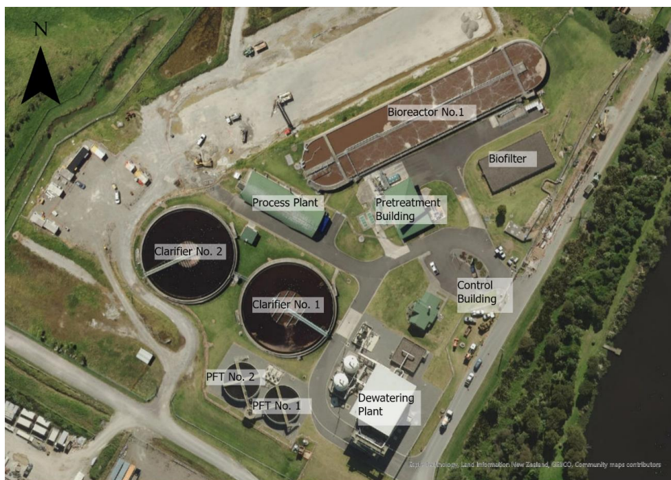
Figure 4. Aerial image of Te Maunga wastewater treatment plant with labelled components.
