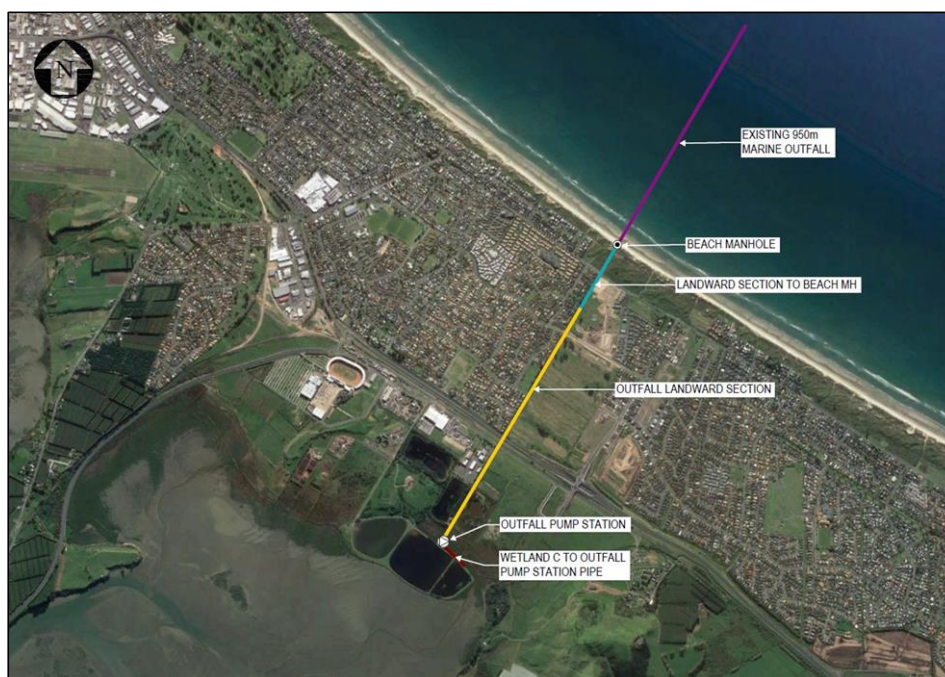
Figure 6. Outfall pump station and outfall pipe. Colours representing the different sections of pipe.
