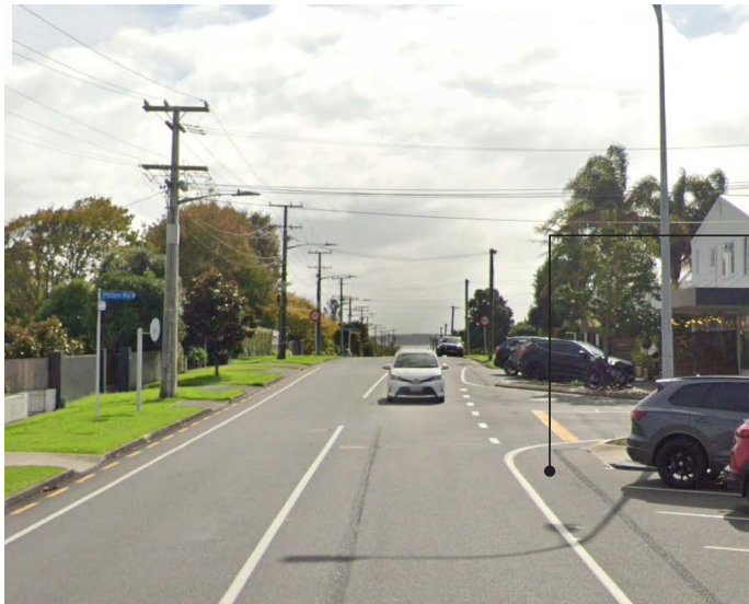
Informal crossing at Milton Road has poor sightlines due to car parking blocking visibility. Children regularly cross this busy intersection whilst having to consider fast moving traffic and reversing vehicles
