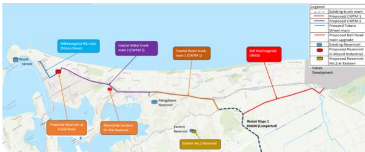
Figure 2: Eastern Corridor planned and proposed Water Supply Projects
